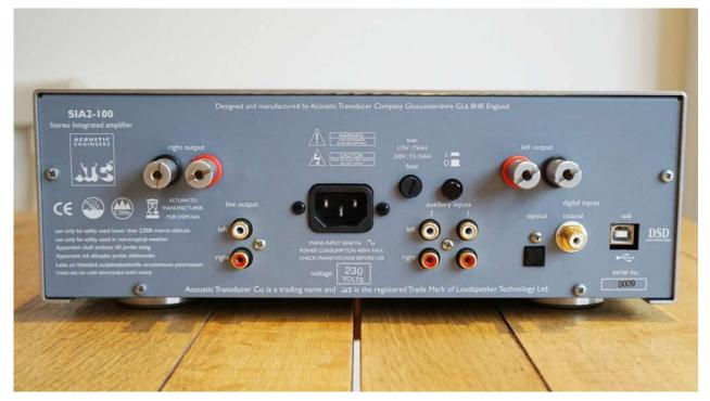
Two sets of multi-way speaker binding posts join two pairs of analogue RCA inputs, three digital inputs and analogue pre-outputs
