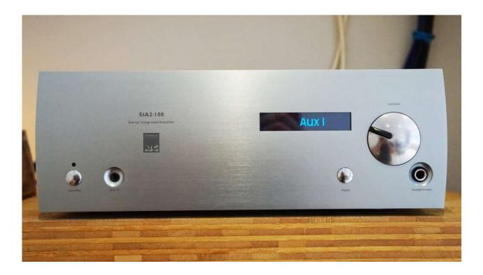
Just a trio of controls for power, source and volume plus an LED screen keep the ATC's front panel pure and simple. Headphone jack and analogue input are practical extras
