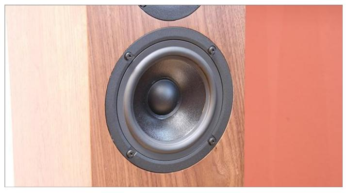
Xavian NEOX2 be able to tolerance -3 db play in their dimensions decent range 42-20 000 Hz for. The lowermost converter operates between 42-250 Hz, medium from 250 to 2600 Hz and then handles the rest tweeter reproduction. Speakers are declared as 4 ohm characteristic sensitivity and achieves relatively high 89 db / 2V / m.
