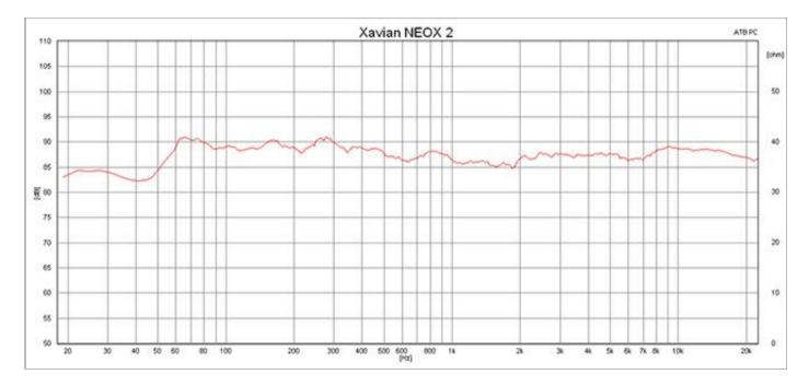
The frequency response curve is simply exemplary. Real onset of reproduction fully meets the stated 42 Hz, while the indication of the extent to 20,000 Hz, as measured by the very conservative. Considering that it is a classic top heading does changer "hold" without a drop in energy apparently beyond this level. The chart also shows slightly, but really only very slightly richer deeper tones up to about 300 Hz. In the context of the speakers 40-50 000 - but the curve is "straight as a bullet."
