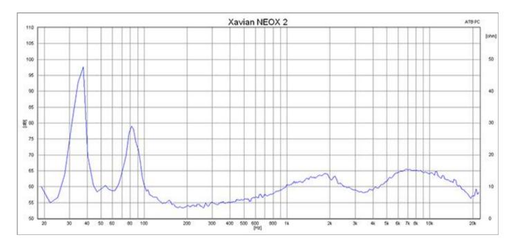
The impedance curve is also relatively mannered, never falls to dangerously low levels. Over the top somewhere near the 15 Ohm not the management NEOX2 no problem, the curve is simple and fast transients big differences. Artifacts below 100 Hz oscillations are caused by operational amplifier in your sound card, not by the speaker.
